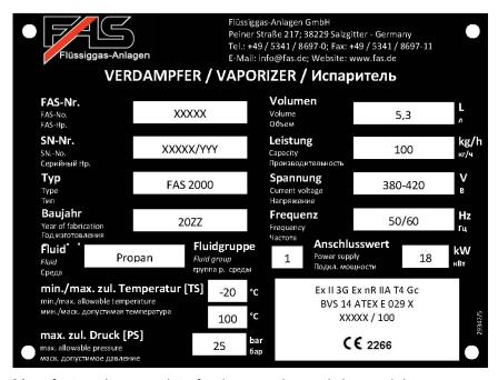
Manufacturer's nameplate for the vaporizer unit (example)
